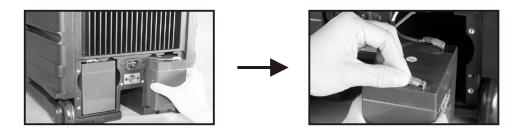
3. Connect red-color wire and black-color wire. Ensure the red color cable is positioned on top, near the "+" terminal. Connect a 3rd cable (red color) to the terminal socket only for Left Side Compartment when replacing with MB-80.
