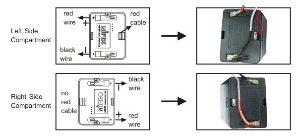
4. Insert connected battery into left and right compartment. Fasten the screws once it is covered by steel protection cover plate.
