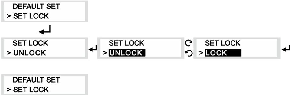
1. Rotate the rotary control knob to select "SET LOCK" then press the knob to enter.
