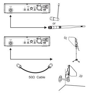
(C) MIPRO AD-90S high power splitter, or AD-90A high power amplifier, can be installed to greatly increase transmitting range and coverage to reduce signal dropouts.
