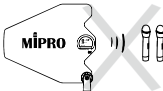
Fig. Right: × Incorrect, antenna facing backward
